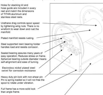
Frame is made from cold rolled steel sheet instead of hot rolled angle. Hot rolled is rough and includes pits so it is difficult to get a proper coating. Cold rolled steel sheet is smooth and non porous so the powder coating will better resist rusting.
