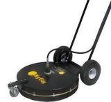
The Lil Big Guy: Powder coated aluminum housing, Over-sized, self-lubricating twin thrust bearings, 10" pneumatic tires, 4" caster, crafted with stainless steel and aircraft aluminum, 212°F, 4-10 GPM, Dimensions 24"x44"x12".
